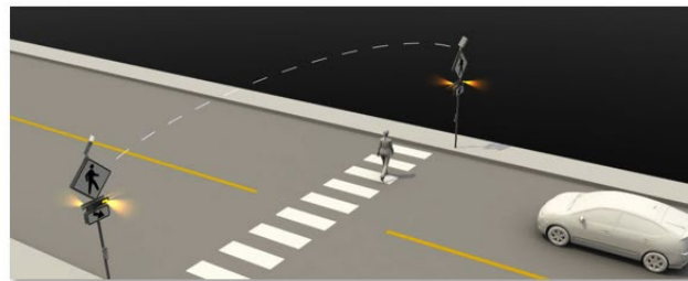
Figure 79 PHB and RRFBs Proven Safety Countermeasures Examples
