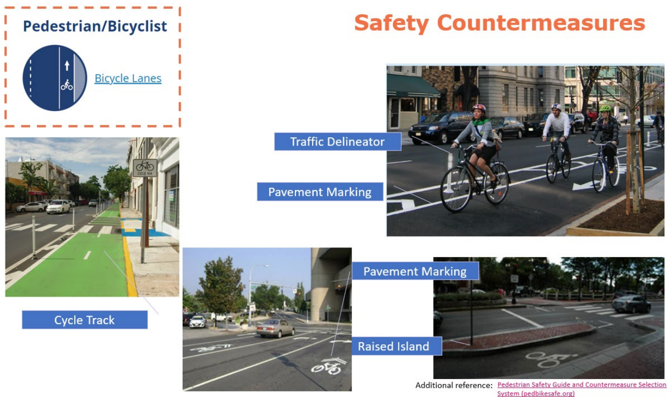
Figure 75 Bicycle Lane Proven Safety Countermeasures Examples
